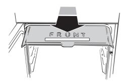
Remove the oven roof by sliding it forwards.
